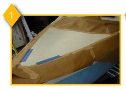
When a section may not have a good straight edge, you can secure the FLEX-MOLD and start process in a more suitable place.
