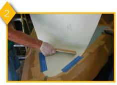
Press FLEX-MOLD down with a squeegee, apply gelcoat and start process.
