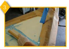
After initial squeegee out, press squeegee down to hold a seal as you pull off the tape.
